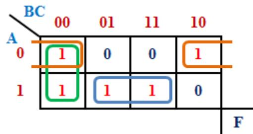
$$F = \bar{B}\bar{C} + AC + \bar{A}\bar{C}$$
