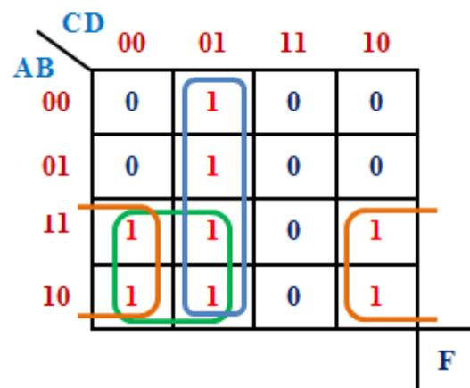
$$F = A\bar{C} + \bar{C}D + A\bar{D}$$
